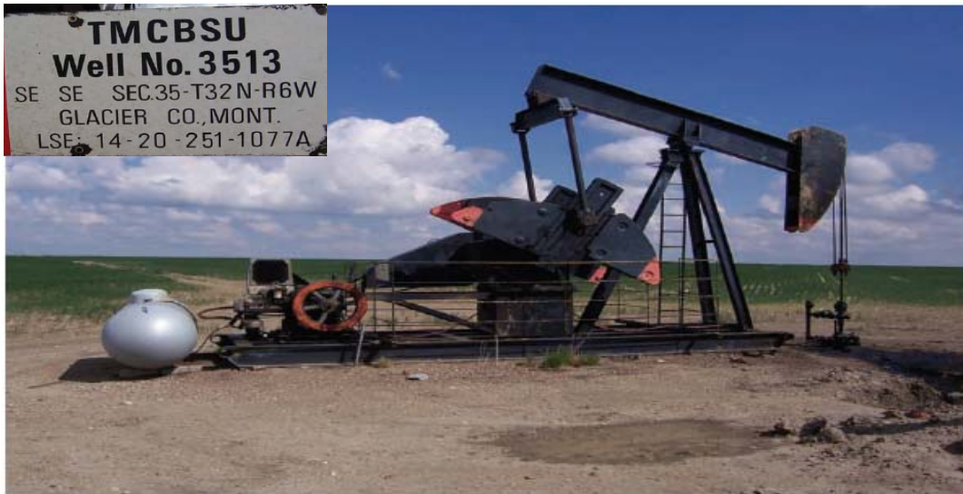
Figure A 7.7: Skid Mounted Pumping Unit.
