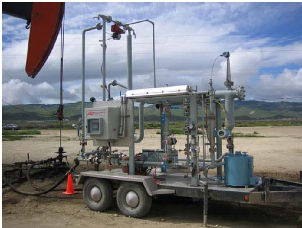
Figure A 7.6: Portable test unit that enables single-well tests.
